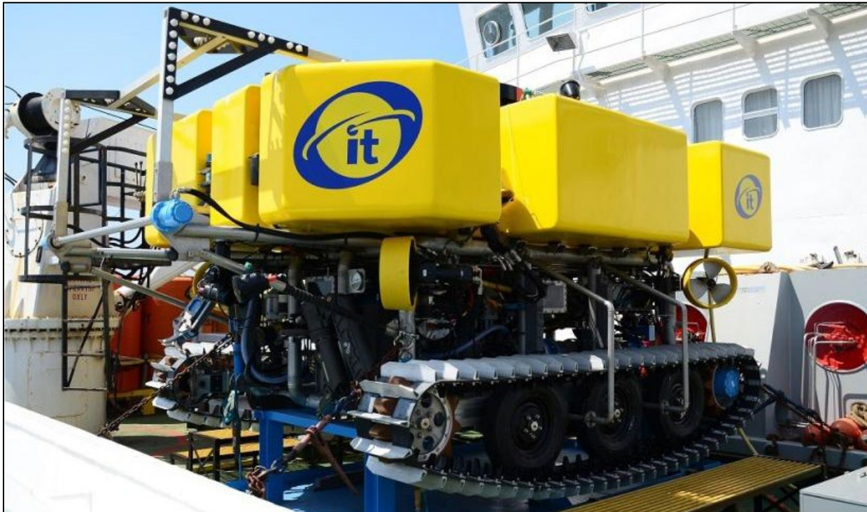
Photograph 5: ROVJET 207 (Manufactured by International Telecom)
