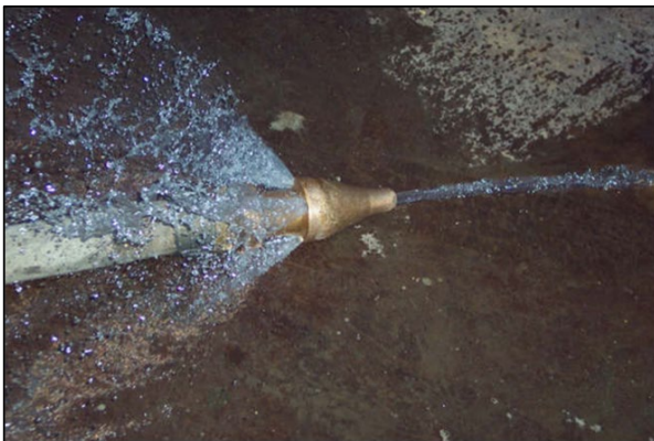
Figure 7. Photo and graphic examples of diver jetting.
