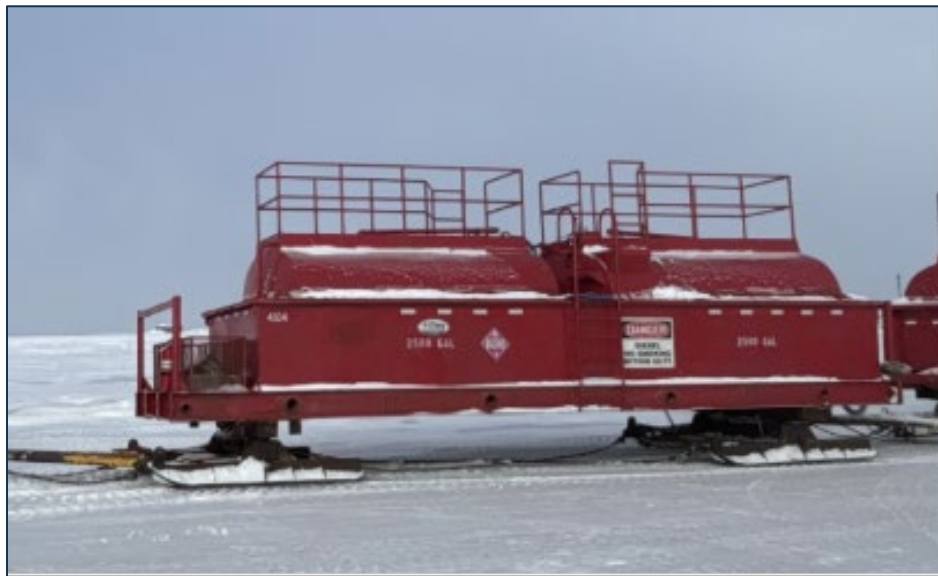
Figure 4: Mobile fuel sleigh contains two 5,000-gallon double-walled tanks
