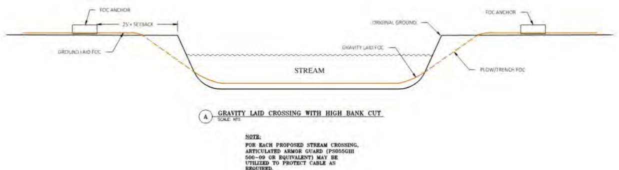
Figure 6: Typical gravity lay fiber cross-section for small stream crossings with steep banks.
