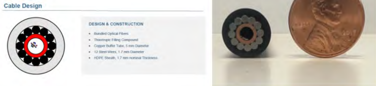
Figure 2: Fiber optic cable specifications.
