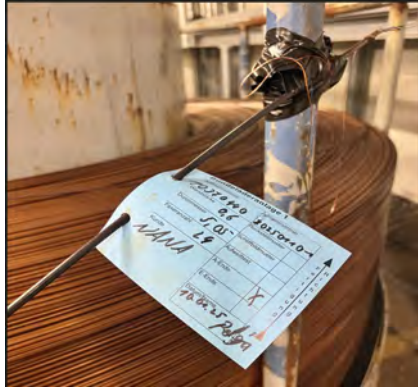
Fiber Inside Copper Tubing Before Armoring
