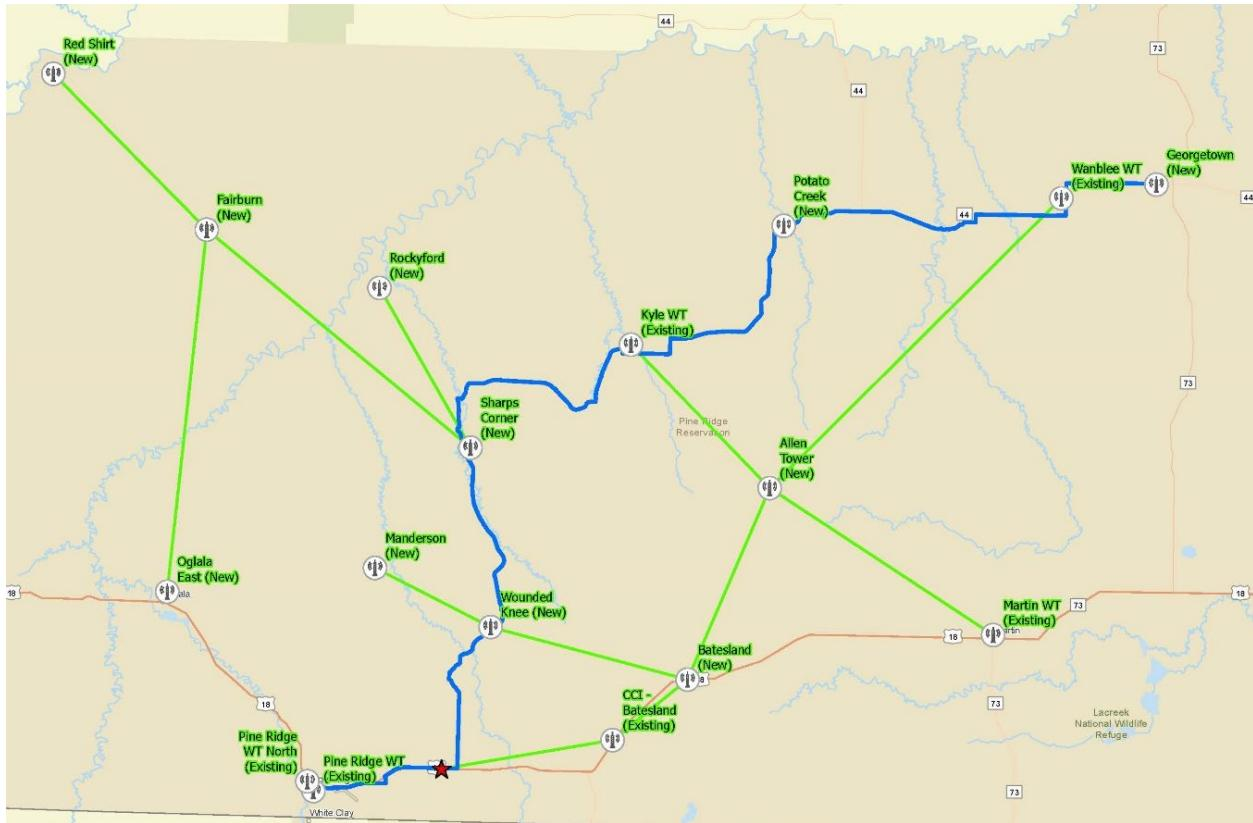
**Note:** In the image above, new and existing tower and pole locations, as well as microwave backhaul links, are highlighted in green. The mainline fiber route is highlighted in blue, and the network Point of Presence (POP) is marked with a red star.
