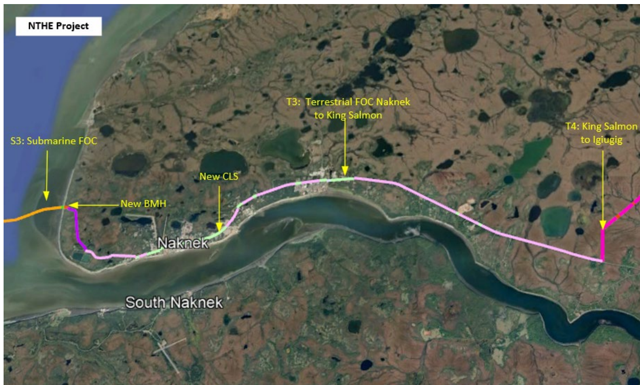
Figure 16: Naknek Landing Point – BMH location
