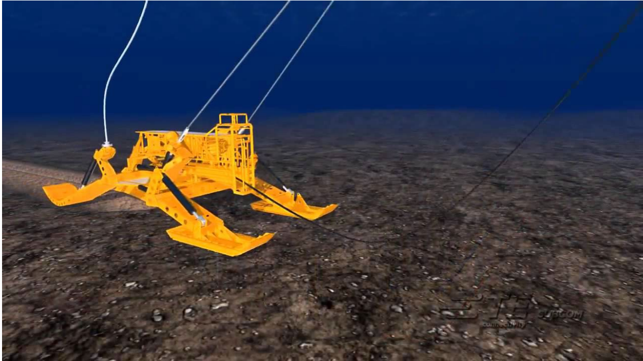
Figure 4. Sample fiber optic cable undersea plow (TE Services 2025).
