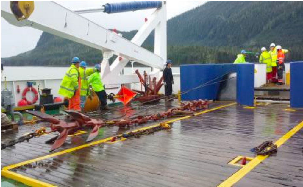
Figure 3. Example marine grapnel on the deck of a cable vessel (48 North 2025)
