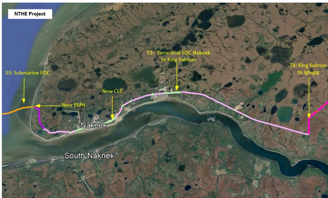
Figure 16: Naknek Landing Point – BMH location
