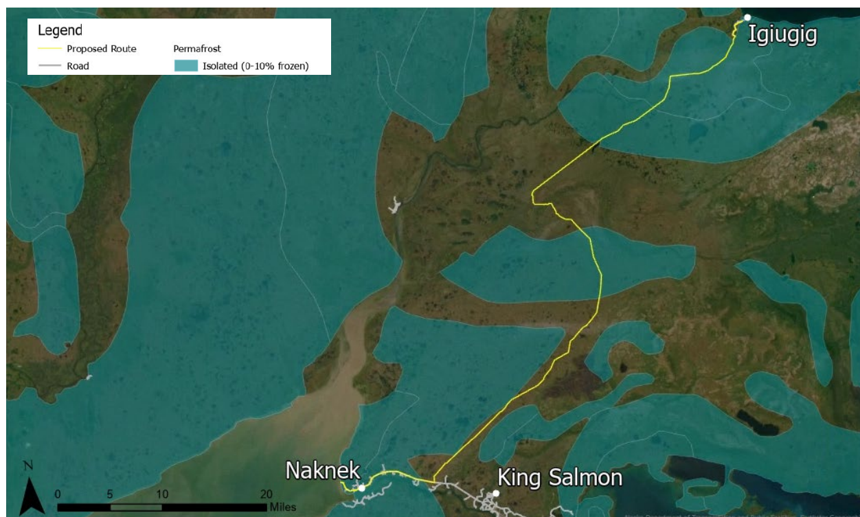
Figure 9. Permafrost Along the Naknek to Igiugig FOC Route
