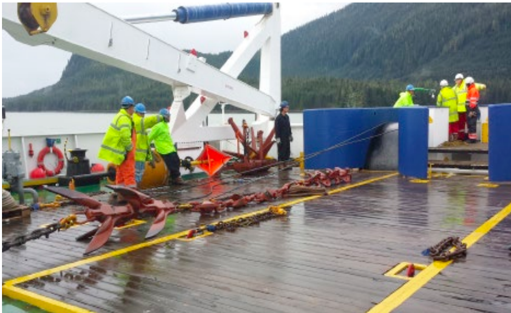
Figure 7: Grapnel on the deck of main lay cable vessel
