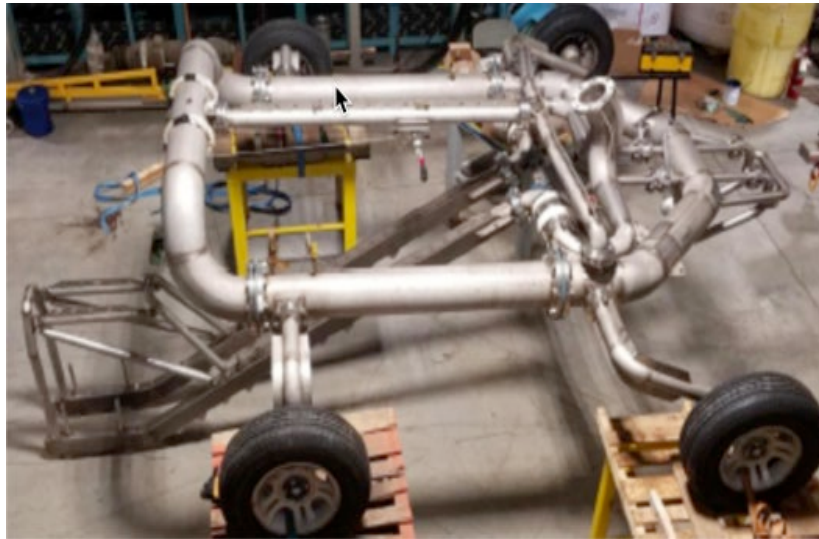
Figure 9: Typical jet sled
