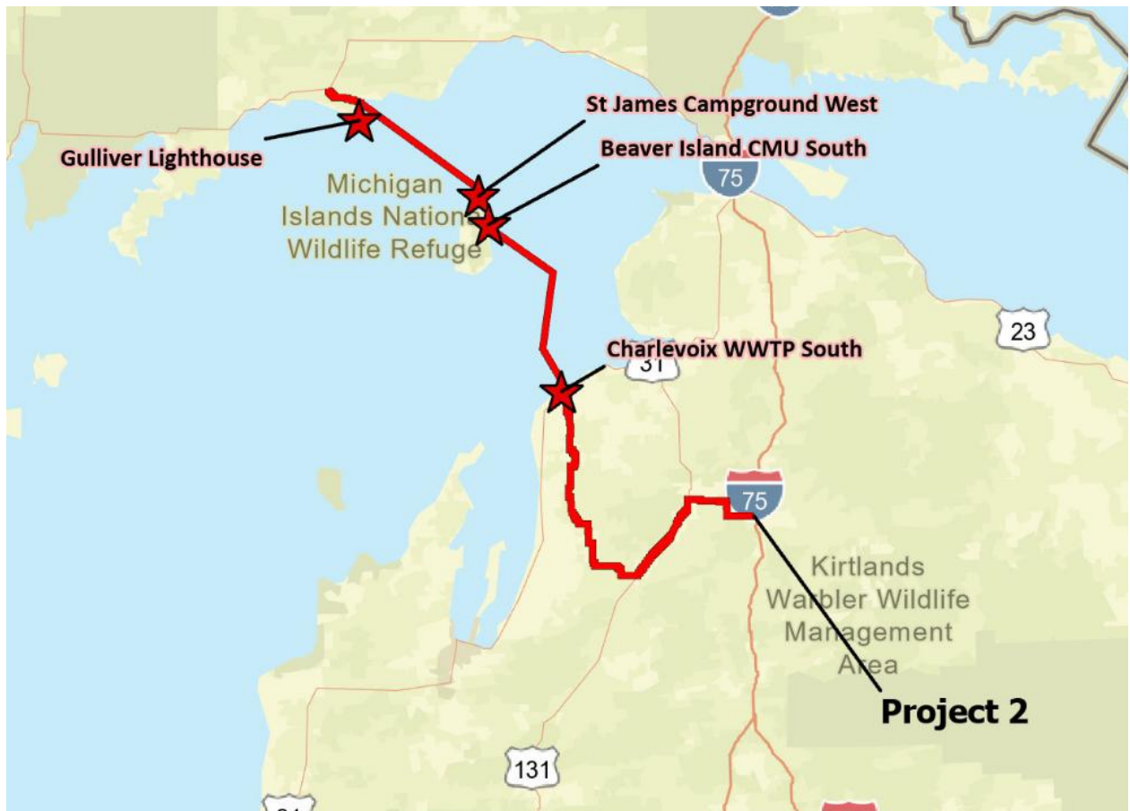
Figure 3. Project 2 Fiberoptic Cable Route
