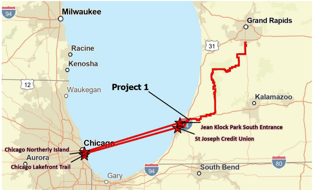
Figure 2. Project 1 Fiber optic Cable Route
