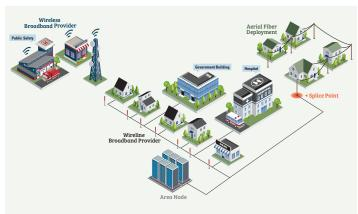
These networks are often optical fiber networks in which the cables are either buried in underground conduit or strung on utility poles through an aerial deployment. In remote rural areas, such as tribal lands, or across difficult terrain, equipment for microwave and wireless broadband networks are mounted on towers so that broadband signals can reach homes, businesses, institutions and government facilities.
